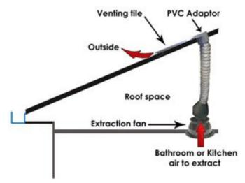
Available for Concrete tiles and Corrugated/Colorbond metal roofing
